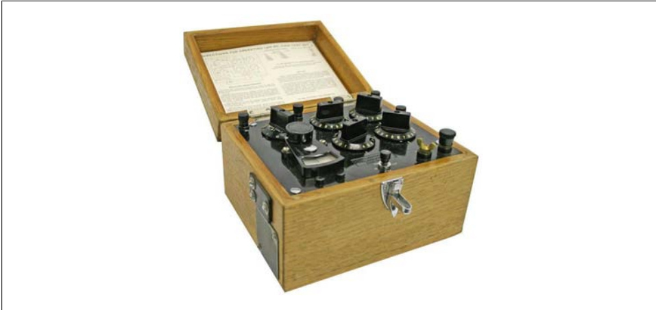
Figure 6-5. Vintage Leeds and Northrup Resistance Bridge Test Set
